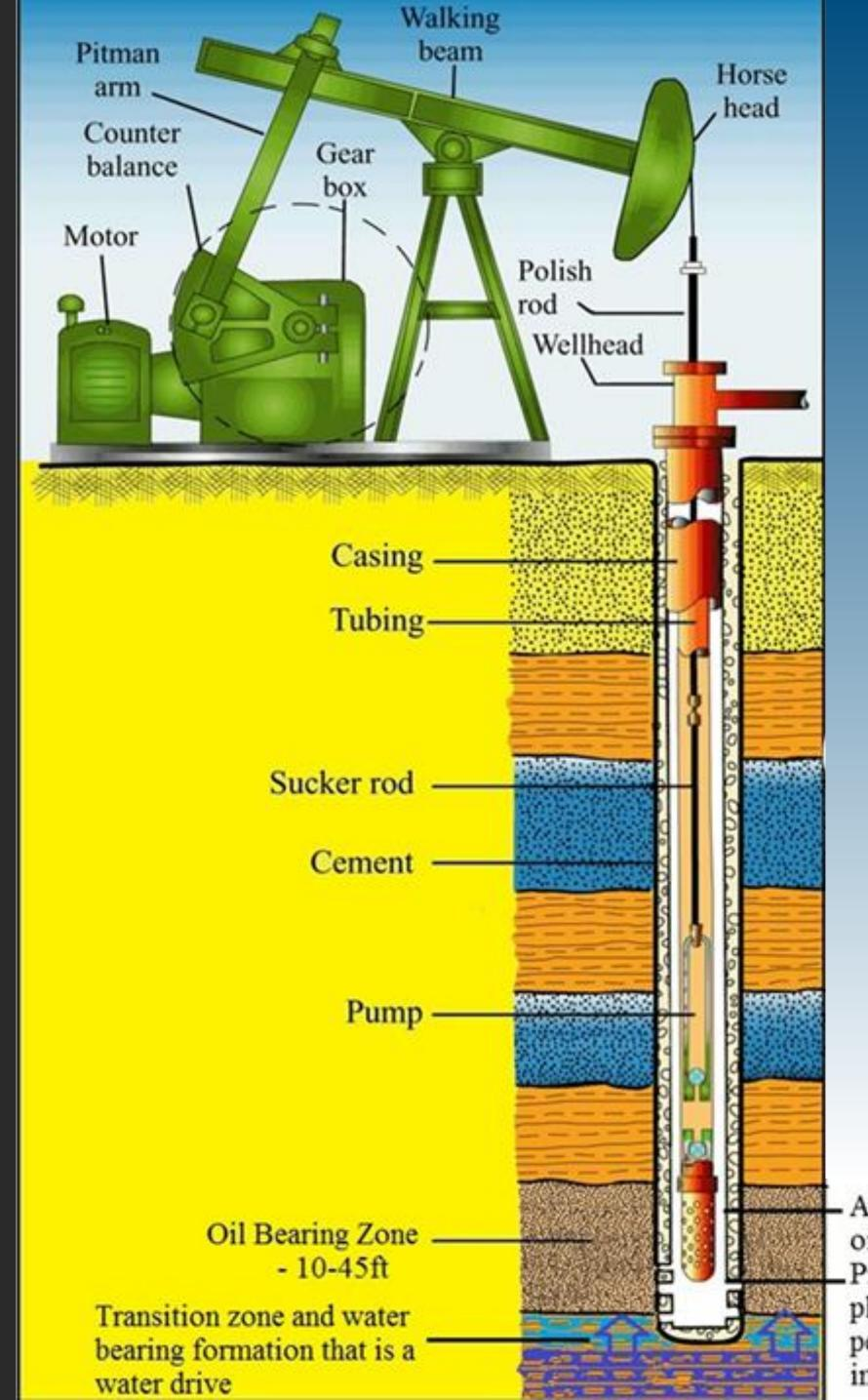
Area of Future Perforations, in oil bearing rock Previous Perforations, Manual plug will be placed above OLD perfs, to seal off water intrusion into the well bore
